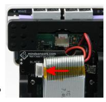
Fully charged up new battery will measure about 8.2 volts.
